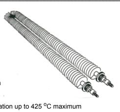
The completed assembly is finished in a high temperature aluminium paint for operation up to 425 °C maximum sheath temperature. Mounting bushes are 3/8" B.S.P. x 15 mm long.
